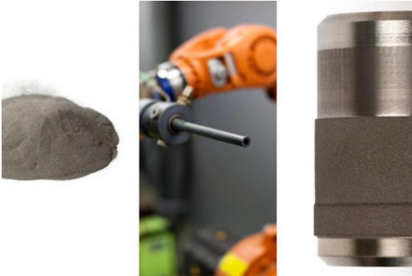
*Figure 20.4* Refining of steel parts using thermal spraying processes by Putzier.
